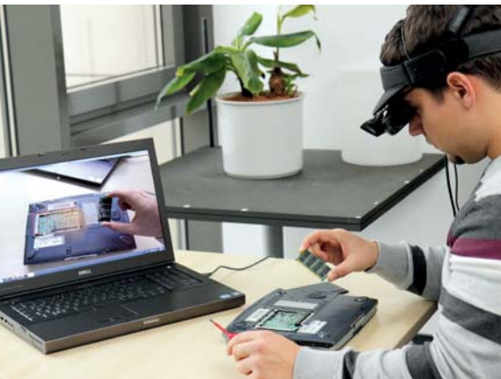
The image on the notebook shows what the AR manual user sees through the head-mounted display
