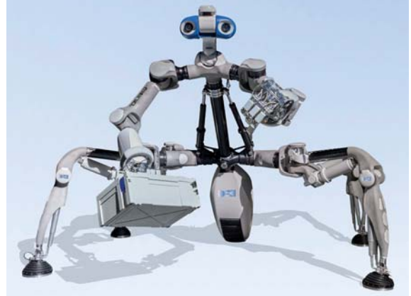
A biomimetic walking robot that resembles a praying mantis
