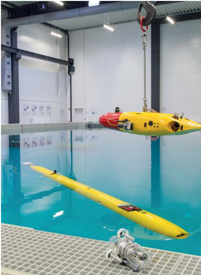
Autonomous underwater vehicles (AUVs) at DFKI Maritime Exploration Hall in Bremen
