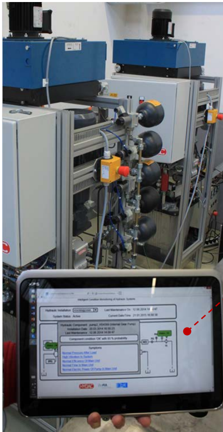
Mobile client for monitoring hydraulic test benches
