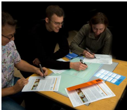
Figure 2. Co-located collaboration with CoScribe. Each user has a personal pen to interact both with printed media and digital information on a tabletop display.
