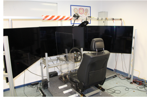
Figure 2: Setup overview showing our driving simulation with three 55-inch screens, steering wheels, and pedals. We simulate the car’s left door with a plastic barrier beside the driving seat. Sensor cameras are attached to a top beam to simulate their location on the roof of modern vehicles.
