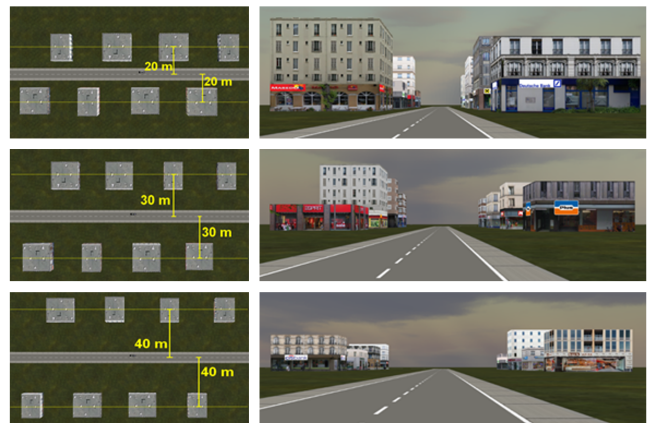
Figure 3: Buildings’ clusters with the three possible lateral building offsets. The Left is the top view, and the right is the driver’s view.
