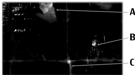
Figure 3. IR camera image, A) Users palm, B) imperfections of the surface, C) Joints of the blocks
