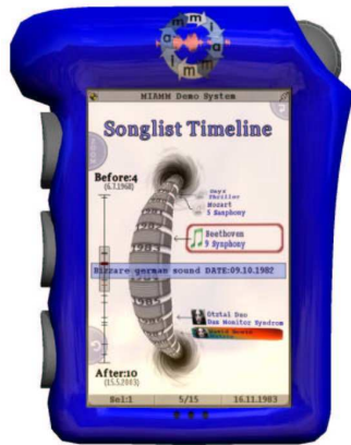
Figure 2: The force-feedback device developed in the MI-AMM project. The display shows a view of a database using a timeline.
