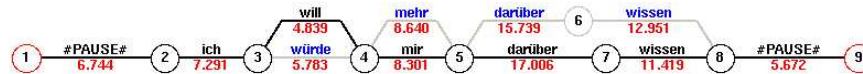
Fig. 4. Word hypothesis graph for “I would like to know more about this”.
