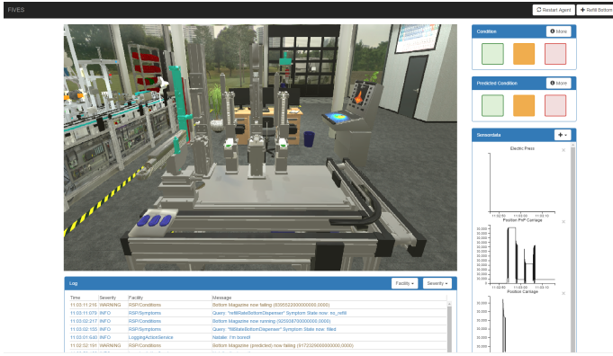
Fig. 6. Smart Factory production module in virtual 3D representation with dashboard containing sensor data and status information.
