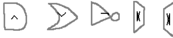
Fig. 3. Gates which are recognized by the system (from left to right): and , or , not , multiplexer , and demultiplexer ; the visual feedback of the system is illustrated in black
