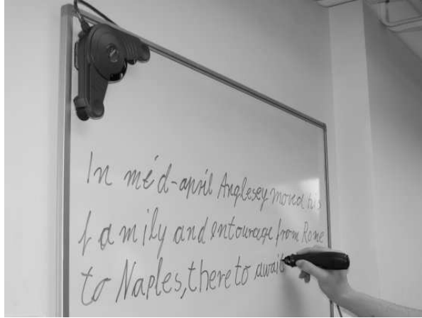
Fig. 3. Recording session with the data acquisition device positioned in the upper left corner of the whiteboard
