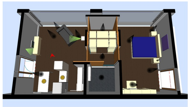
Figure 2. The lights and sliding doors of DFKI's Ambient Assisted Living Lab (BAALL) in Bremen are synchronized with the 3-D model. They can also be interactively controlled from the model.
