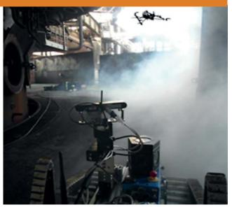
**Semi-autonomous ground and air robots exploring the terrain.**Photo: tradr-projecteu
