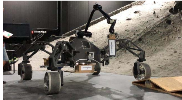
Fig. 10. Preliminary integration tests performed at DFKI with a mockup of the P-APM attached in folded configuration under SHERPA-TT body and a mockup of the A-APM attached to the tip of its robot arm manipulator. (credit: DFKI GmbH)
