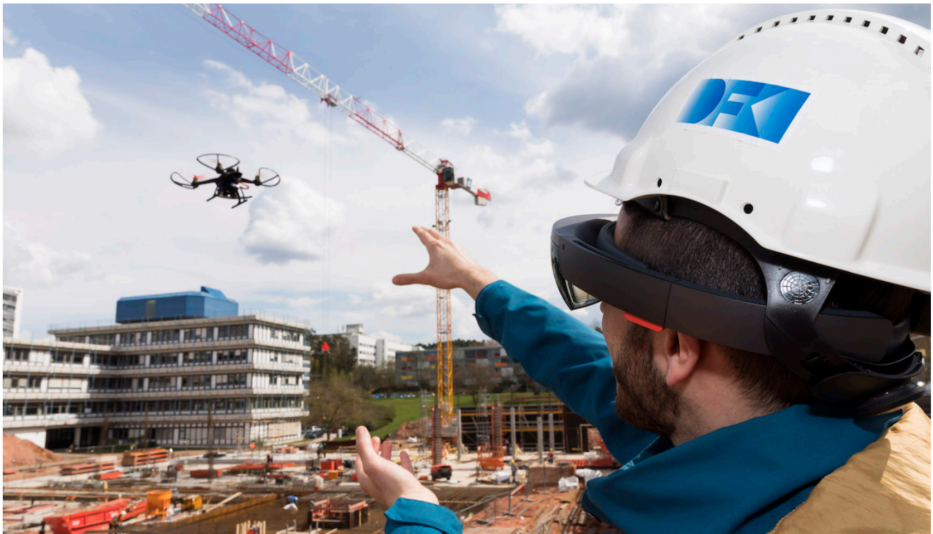
Figure 1: In the project's vision, construction workers have access to and can intuitively interact with digital information, e.g. plans, instructions, etc. Meanwhile intelligent sensors capture the progress and state of construction in real time. Photo: DFKI
