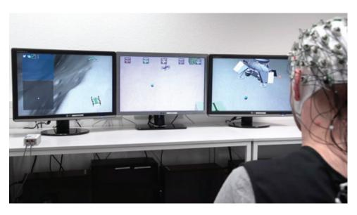
**Figure 14.13** Video: Virtual multi-robot control in 2D using a multi-PC system supported by embedded brain reading. https://www.youtube.com/watch?v=zeFp\_JBSBxA
