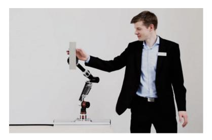
**Figure 14.2** Video: The COMPI arm: compliant trajectory tracking via model-based control allows safe human-robot interaction. https://youtu.be/mDODMNMC5zc.
