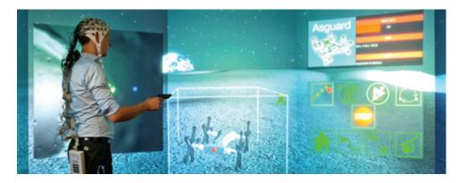
**Figure 14.12** Immersive virtual 3D multi-robot control using a CAVE. Figure courtesy of [Kirchner and Drechsler 2013].
