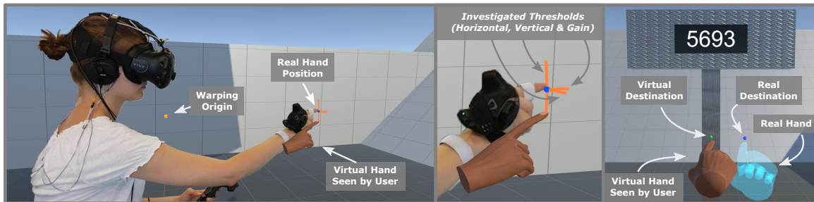
Figure 1: Left & Center: Hand redirection in VR. A warping algorithm displaces the rendered virtual hand from the real hand. According to our results, the virtual fingertip can unnoticeably be displaced to any point along the orange lines. Right: The Vis-DT condition in our experiment. The user reaches for the green target sphere with the displaced virtual hand while reading out the displayed number. The real hand location is added for illustration.
