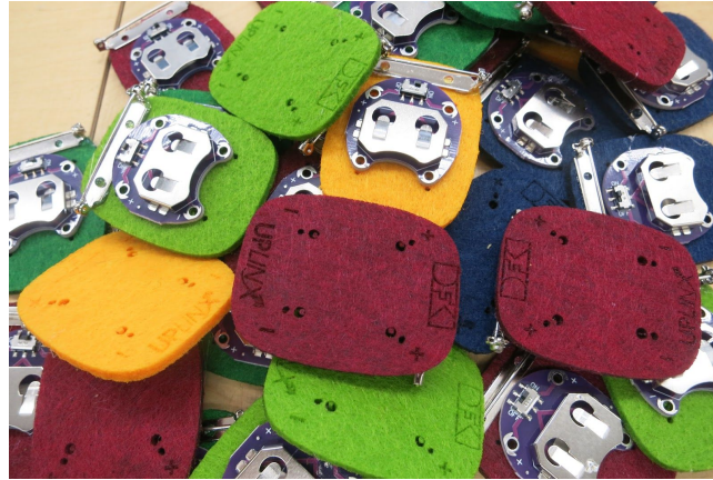
Figure 2: Laser-cutted felt with coin cell battery holder for the hands-on exercise
