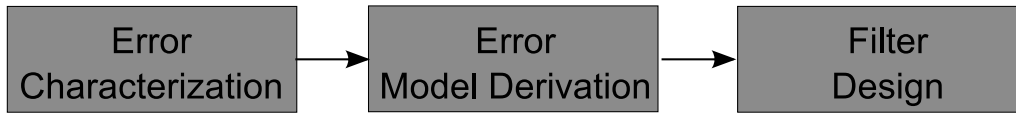
Figure 3.1: Schematic representation of the End to End (E2E) approach for AHRS design. Figure adapted from Hidalgo-Carrio et al. (2012b).
