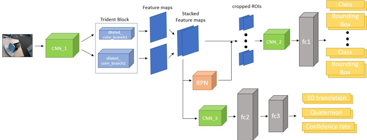
Figure 4: Our proposed architecture based on a modified TridentNet with an additional branch for pose estimation. The details of the network are summarized in the sec. 6.2
