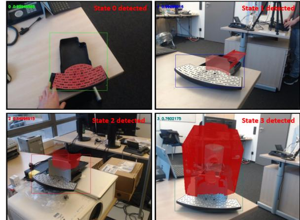
Figure 1: Proposed AR Assembly application using object state and pose estimation. The missing component to move to the next assembly state is visualized.
