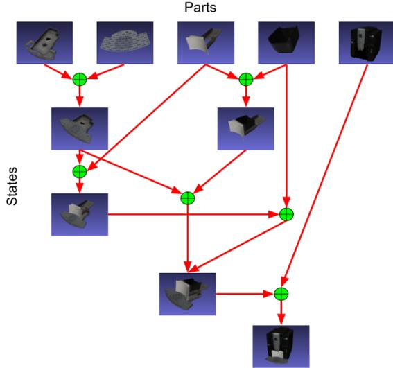
Figure 2: Object State Graph example. Single components can be combined in different ways to assemble the object. The example of a coffee machine is shown here.
