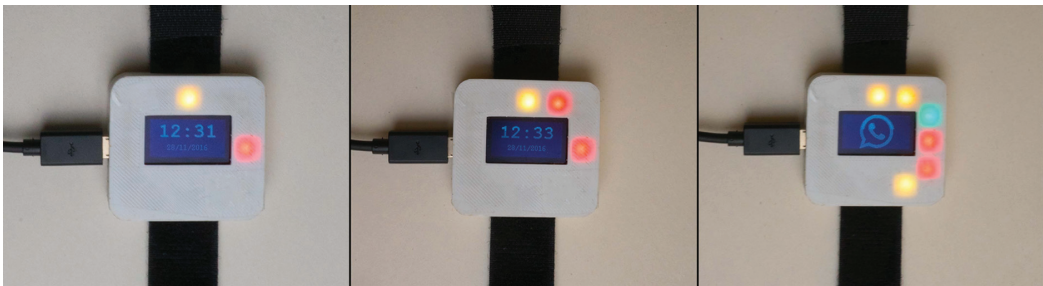
Figure 3. Possible visualizations making use of color, spatial arrangement, and showing additional information on the low-resolution display
