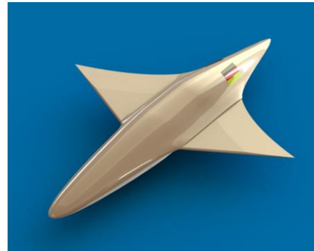
Fig. 10. Concept proposal of nanoAUV for Europa moon ocean and ice research.
