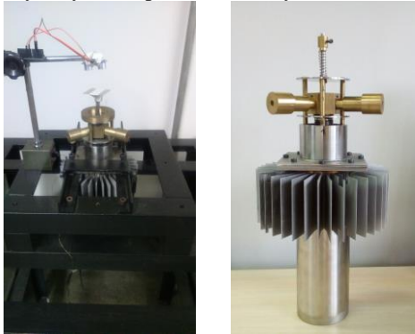
Fig. 5. Brazilian Stirling engine nested in its text cradle and alone for better visualisation.
