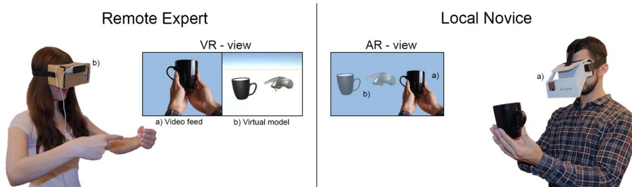
**Figure 1:** The expert (left) wears a Google Cardboard with a Leap Motion Controller attached, allowing her to interact with a virtual proxy object (b) and to see a shared video-feed (a) from the novice. The novice (right) wears an Ayzon Augmented Reality device. He sees the expert's virtual proxy object and her captured gestures (b).
