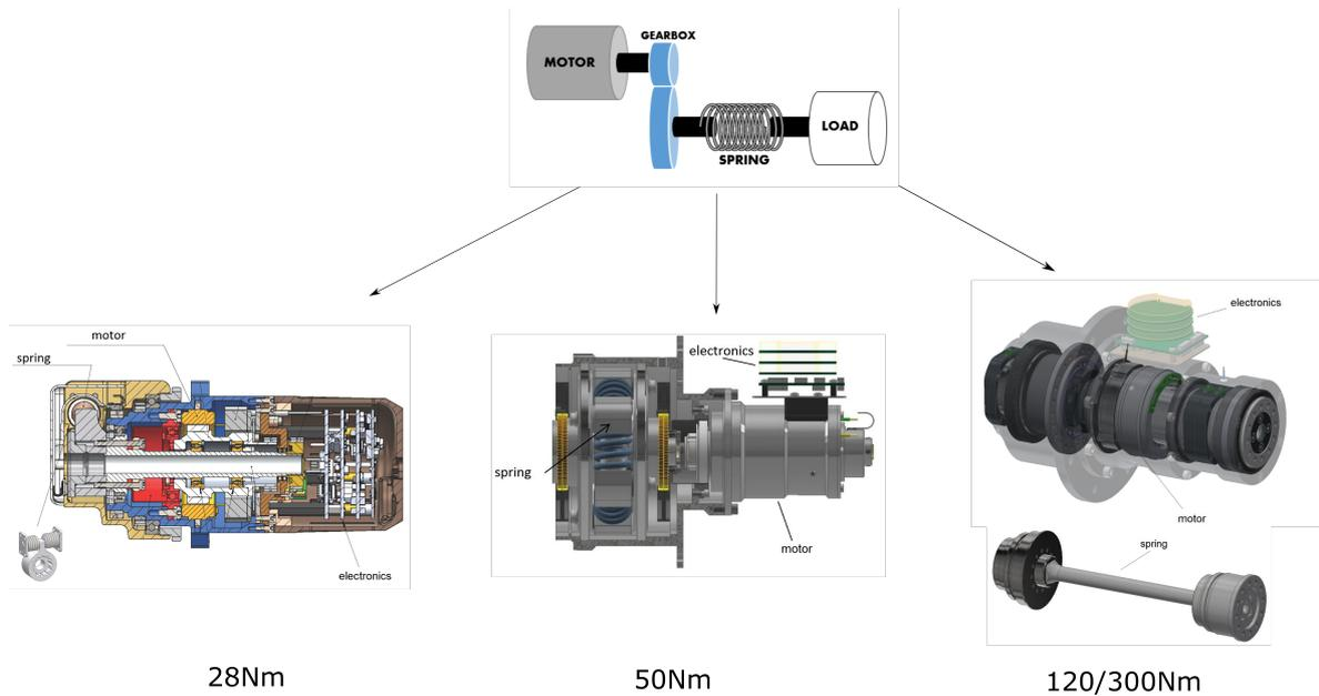
**Figure 2.** Relative position and type of the spring for the developed force-sensing serial-elastic actuators (FSEA). Type of spring for each actuator: *left*: Disc springs (28Nm actuator), *right*: coil springs (50Nm actuator), *right*: torsion bar (120Nm and 300Nm actuators)
