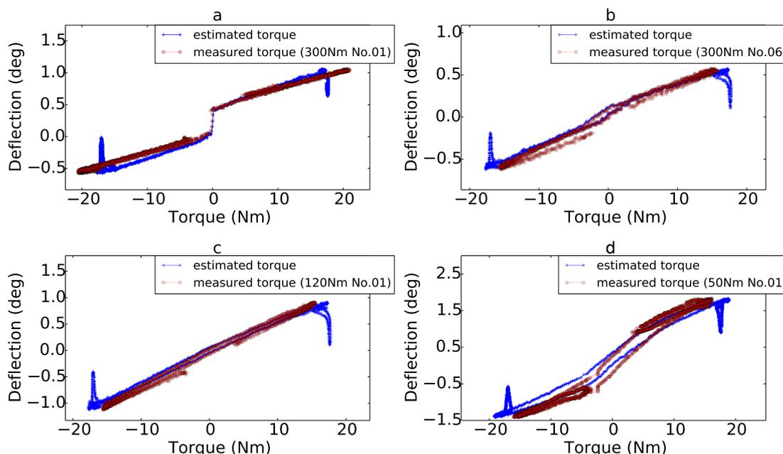
**Figure 9.** a: Results of the torque estimation on 300Nm actuator No.01. b: Results of the torque estimation on 300Nm actuator No.06. c: Results of the torque estimation on 120Nm actuator No.01. d: Results of the torque estimation on 50Nm actuator No.01.
