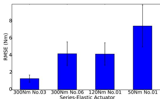
**Figure 10.** Root Mean Square Error (RMSE) and standard deviation of the transfer from model 300 Nm No.03 to three other actuator types.
