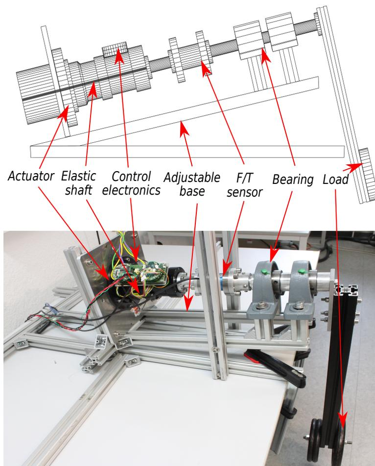
**Figure 11.** Experimental setup used for spring modeling and validation of the torque control.
