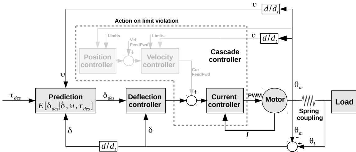
**Figure 6.** Actuator controller structure, composed of a cascade of PI(D) controllers and a model of the spring deflection.
