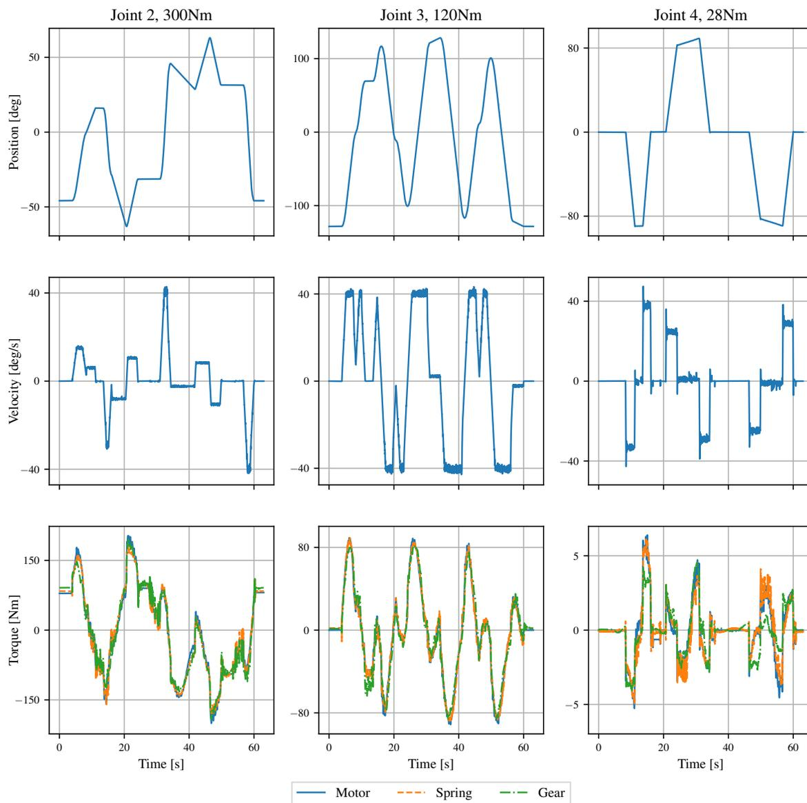
**Figure 14.** Comparison of the different sources of estimated torque (bottom row) for a joint space trajectory (upper two rows); one type of actuator per column.
