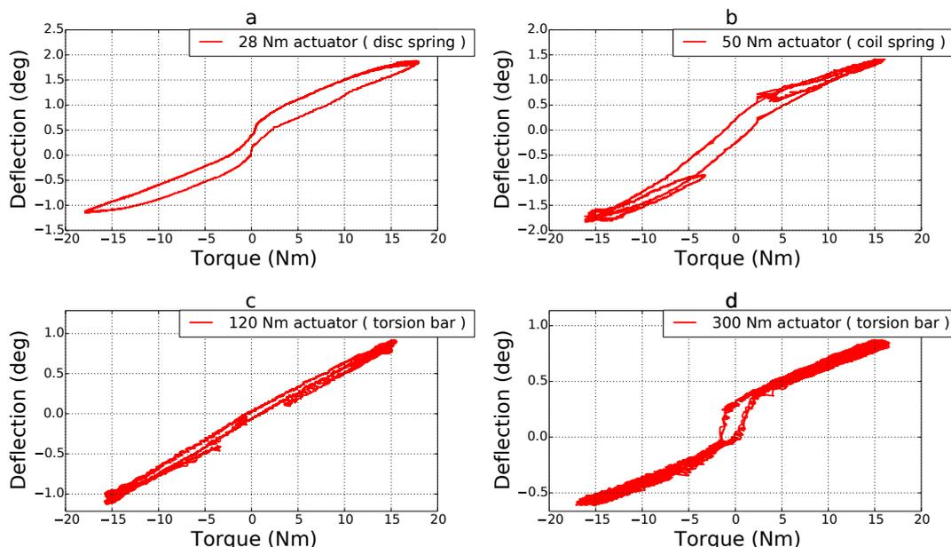
**Figure 7.** Torque-deflection curves of the four actuators. The torques are measured by using an external force/torque sensor and the deflections are calculated as the difference of two absolute encoders at both sides of the spring.
