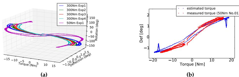
**Figure 8.** Initial result of model transferring from a 300Nm actuator to a 50Nm actuator.
