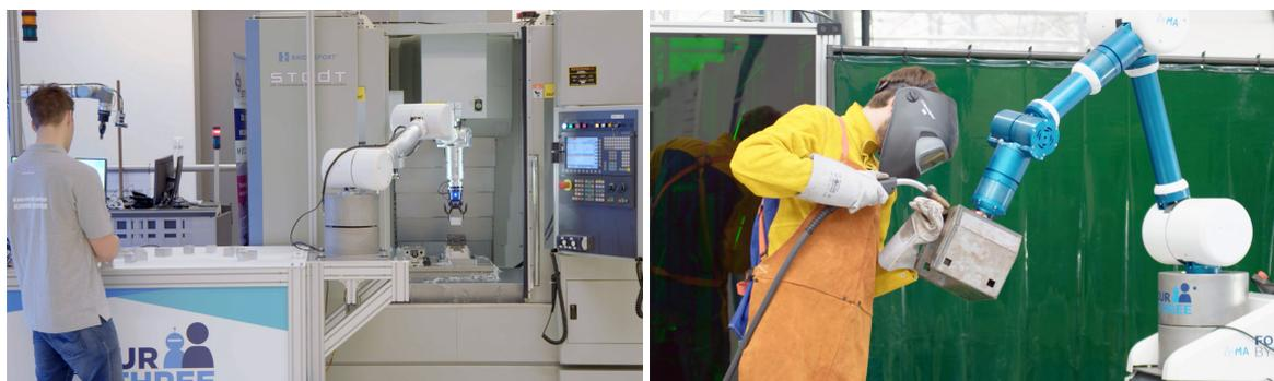
**Figure 15.** Two of the final prototypes at the end-user facilities. *Left:* arm at the company STODT (Netherlands) supporting a person during the loading and unloading of a machine; *right:* arm at the application scenario of the company WOLL (Germany) supporting a person during a welding task by holding and positioning of the workpiece (©FourByThree, permission granted)
