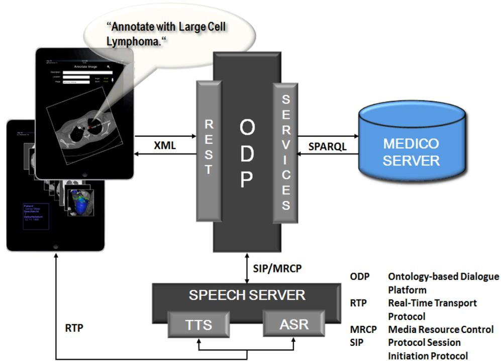
**Figure 1.5** Architecture of the Radspeech System showing components and data protocols, see RadSpeech [2011].
