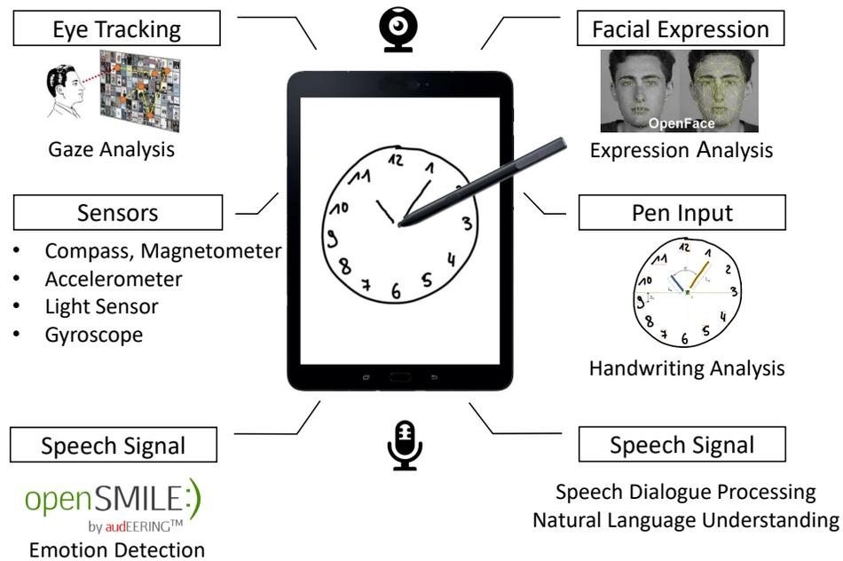
**Figure 1.7** Multimodal-multisensor tablet device.
