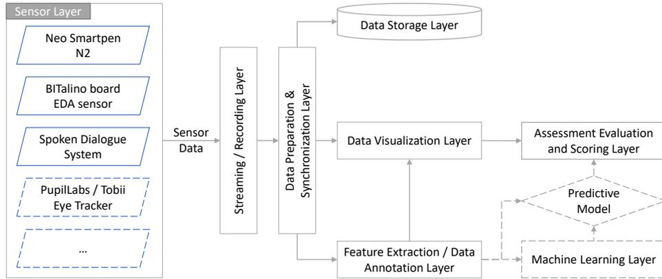
**Figure 1.8** Architecture of the multimodal-multisensor platform used for behavior characterization. Dotted lines indicate work in progress.
