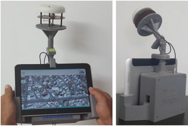
**Fig. 6** LARA system as a prototype
