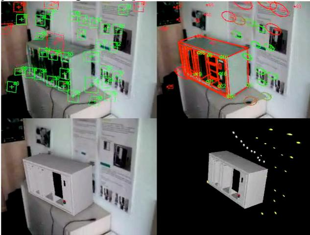
*[image2]: line tracker and KLT, the red lines in the top right part show the fitted line model, the top right shows KLT features. The bottom left image shows the camera image overlaid with the 3d object, bottom left is a visualization of intermediate tracking results (uncertainties of the KLT point*
