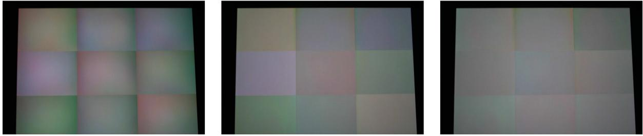
**Figure 6.** A subpart of the wall with nine projectors before any calibration (left), after intra-projector calibration (middle), and after inter-projector calibration (right).
