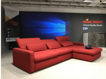
Figure 3: The VR couch configurator booth in the furniture store. The image shows the physical couch providing passive haptic feedback. The projection in the background is used to display the HMD view of the immersed user during the experience.
