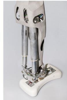
(b) 2 DOF RH5 ANKLE mechanism
