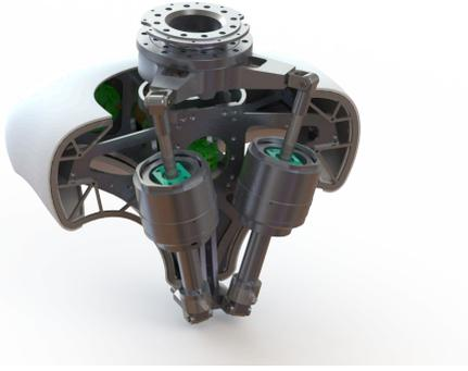
Figure 4.18: CAD prototype of Torso joint
