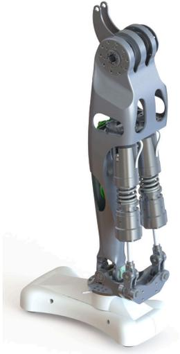
Figure 4.2: CAD prototype of Ankle joint
