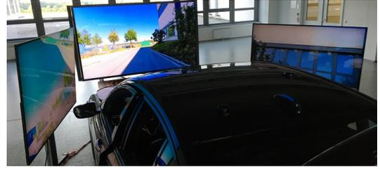
**Figure 5: The simulation setup, playing a route which was prerecorded with  $360^\circ$  camera and edited accordingly.**
