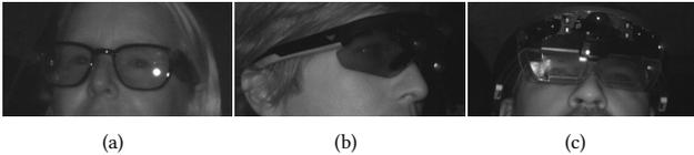
**Figure 4: Example, cropped single IR images of the three other glasses in the recordings: (a) North Focals Generation 1, (b) Everysight Raptor, (c) Hololens 1.**
