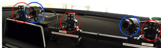
Figure 2: The hardware setup on the car dashboard for the recording. There are three IR-cameras with additional flashers (red). Two marker-base cameras acquire the ground truth poses (blue).
