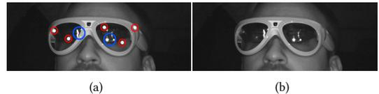
**Figure 7: Example of the Mini Augmented Vision glasses before and after postprocessing. (a) Before postprocessing, where markers are circled red and reflections are highlighted in blue. (b) After postprocessing without markers but visible reflections.**
