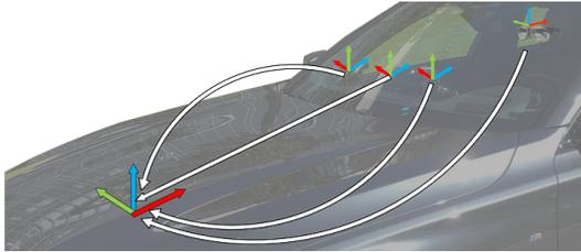
**Figure 3: All coordinate systems and the their transformations. The corresponding  $x, y$  and  $z$  axis are colored red, green and blue, respectively. The common coordinate frame in the front of the car, the three IR cameras pointing towards the passenger and the glasses pose orientation similar to the common coordinate frame are pointed out.**
