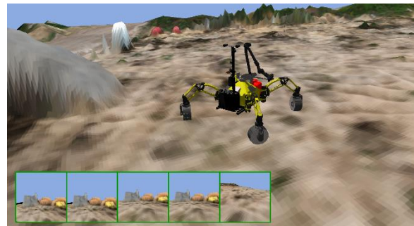
Figure 2: The SherpaTT Simulation includes all sensors available on the rover and the software that controls the simulated rover are the same except for the hardware drivers.
