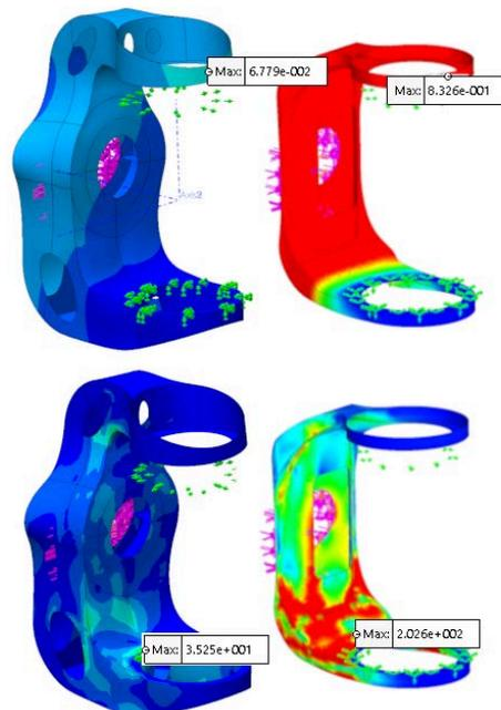
Figure 7: FEA results of hip linkage (left: new; right: old, top: deformation in mm, bottom: van-Mises stress in MPa)
