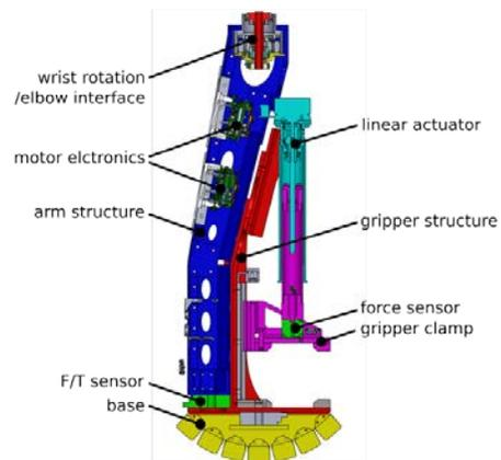
Figure 4: CAD of the new gripper
