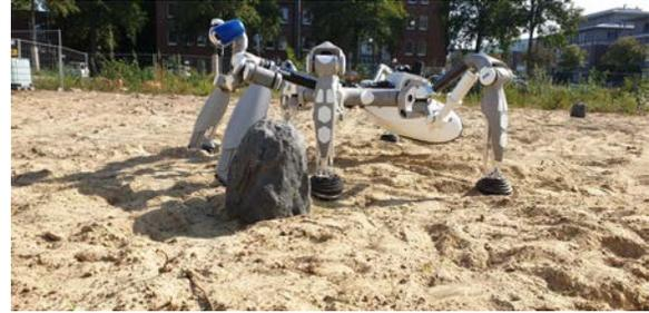
*Figure 12: Mantis outdoor on uneven and sandy terrain performing first tests of CSLAM*
