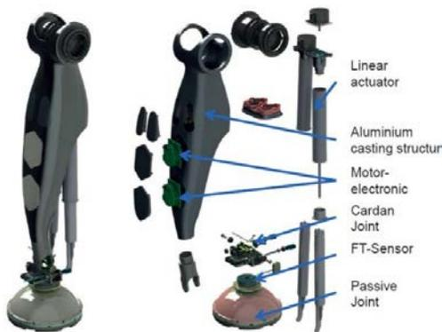
Figure 5: Leg and foot design of Mantis
