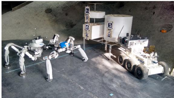
*Figure 11: Mantis, VELES, and the scenario mock-ups (fluid management system, reactor and the housing of the mobile gantry crane) during integration tests in the DFKI space exploration hall*
