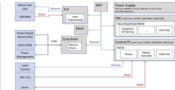
Figure 8: Mantis sensors and electronics
