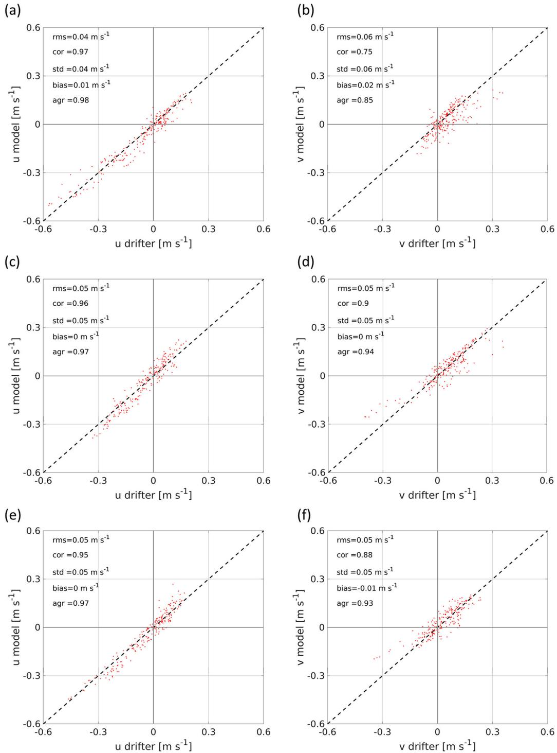
**Figure 4.9.4.** Validation of model surface currents against observations from GPS drifters. Top, middle and bottom panels correspond to drifters 1, 2, and 3, respectively. Left panels: zonal velocity component (u), right panels: meridional velocity component (v). The dashed line is the diagonal and the optimal location of the dots.
