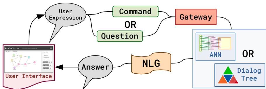
**Figure 4.** Overview of the voice-controlled design component.
