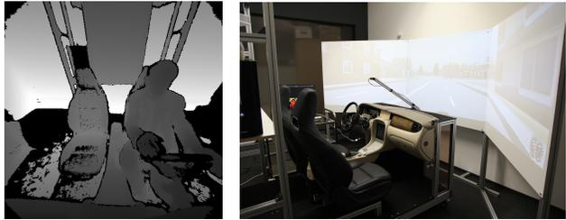
**Fig. 1. Left:** A sample image from the TiCaM dataset, **Right:** The driving simulator setup used to capture TiCaM dataset images.
