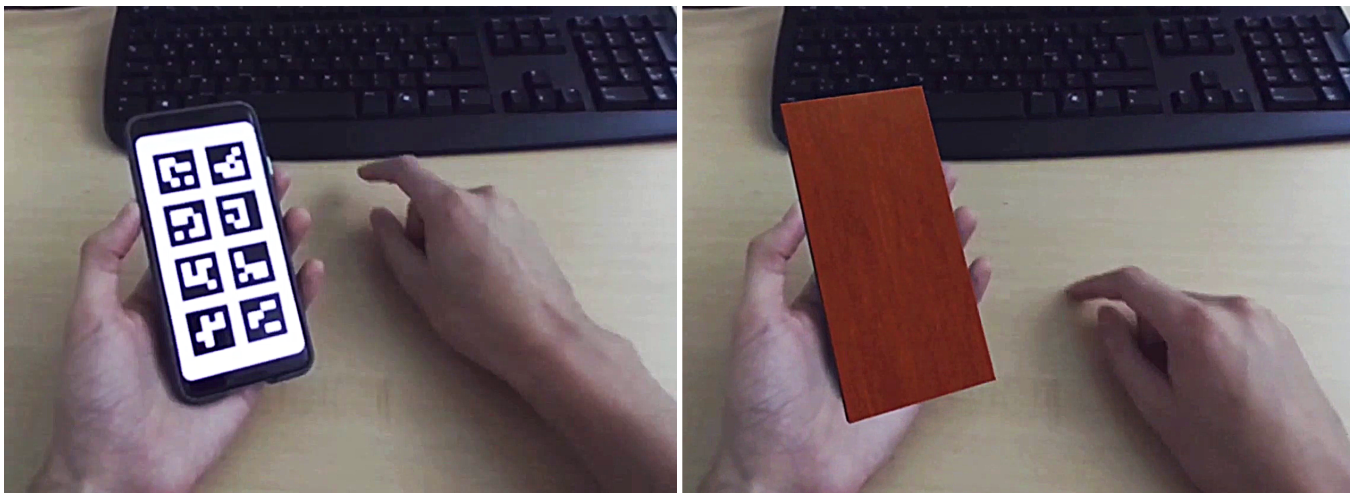
Figure 1: A smartphone is tracked by external camera installed on VR headset. This allows the device to be overlaid with virtual information, rendering the device a smart haptic proxy object.
