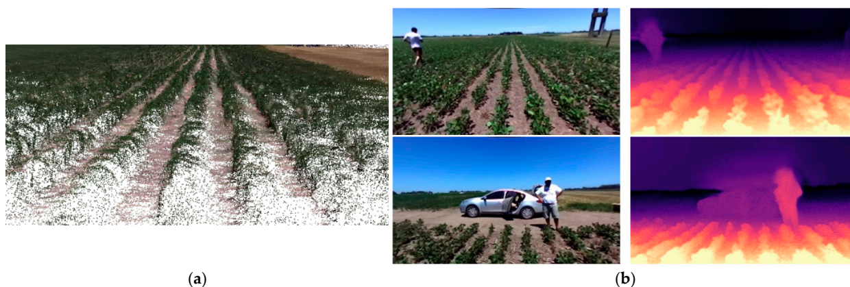
Figure 9. (a) Geo-referenced map (dense point cloud) of soybean field reconstructed from dataset Rosario [26] using SLAM and MVS; (b) scene geometric estimation (depth map) from an unsupervised CNN, which can be used to simulate RGB-D SLAM and boost real-time dense reconstruction [27].
