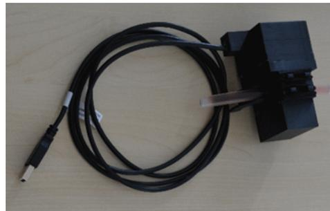
**Figure 8.** Image of the assembled sensor as used in the clinical validation study. Communication and power supply were realized using a USB 3 interface. A short tube segment was inserted to showcase sensor attachment to the CBI system.
