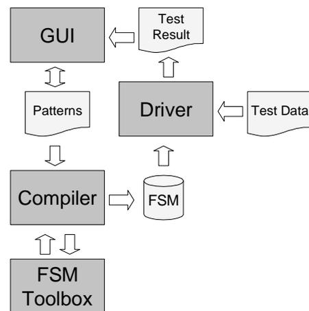
Figure 1. A coarse-grained architecture of the regular compiler.
