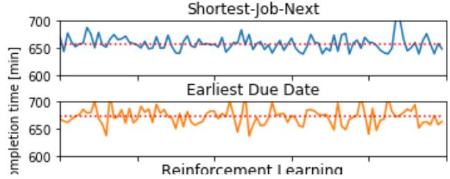
Figure 3 Visualization of the experimentation results for the agent pairs SJN [ $M^{SJN} \times T^{FCFS}$ ] in blue, EDD [ $M^{EDD} \times T^{FCFS}$ ] in orange and RL [ $M^{RL} \times T^{RL}$ ] with their respective mean total makespan  $\bar{C}_{max}$  in red.
