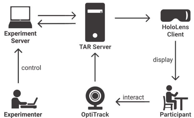
Figure 3: Architecture of the components used for the study.
