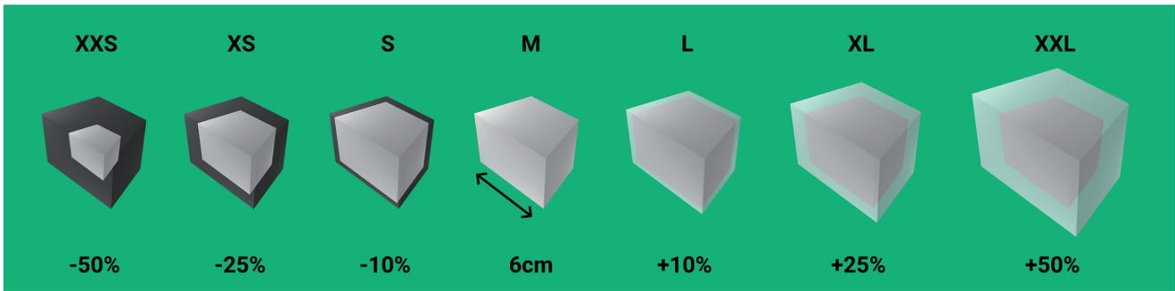
Figure 7: Size variations of the virtual overlays (white) compared to the physical proxy objects (black). Condition M is the base condition with matching size of virtual and physical object.
