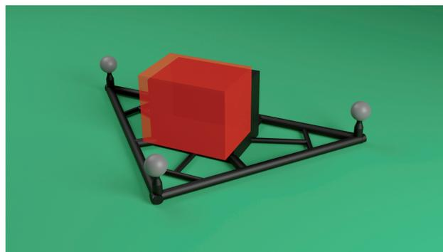
Figure 6: Physical example object for participant's eye calibration. The shifted overlay (red box) is adjusted until it fits the black box.
