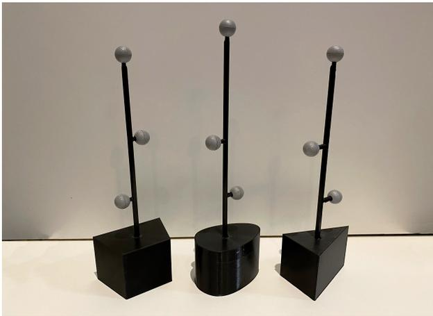
Figure 2: Physical props with attached marker trees on top.
