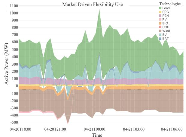
Fig. 5. Market driven flexibility use for low and negative residual load
