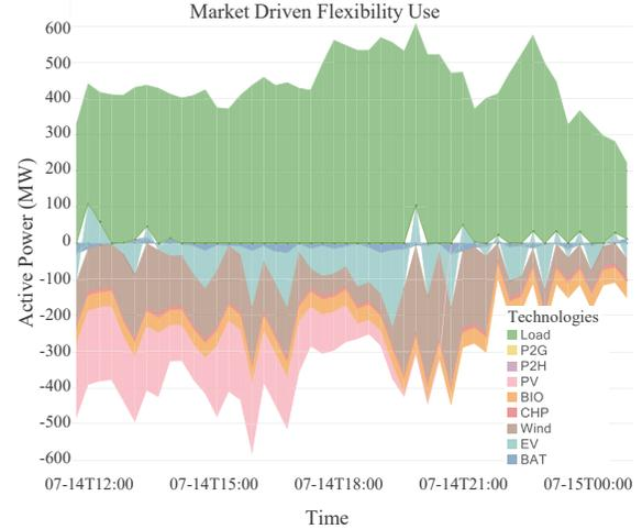
Fig. 4. Market driven flexibility use for positive residual load
