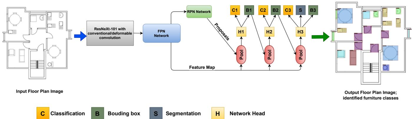
**Figure 4.** The presented framework is based on Cascade Mask R-CNN [15] equipped with ResNeXt-101 [17] backbone with conventional and deformable convolution applied on floor plan images. Modules B, C, and S represent bounding box, classification, and segmentation, respectively.
