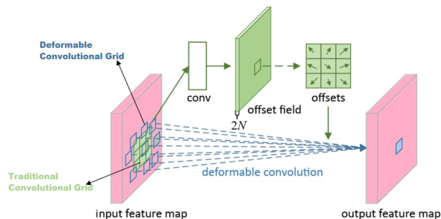
**Figure 5.** Internal working of deformable convolution [16]. The light green grid on the input feature map shows the conventional  $3 \times 3$  convolutional operation, whereas the blue boxes on the input feature map show the effective receptive field of a  $3 \times 3$  deformable convolution.
