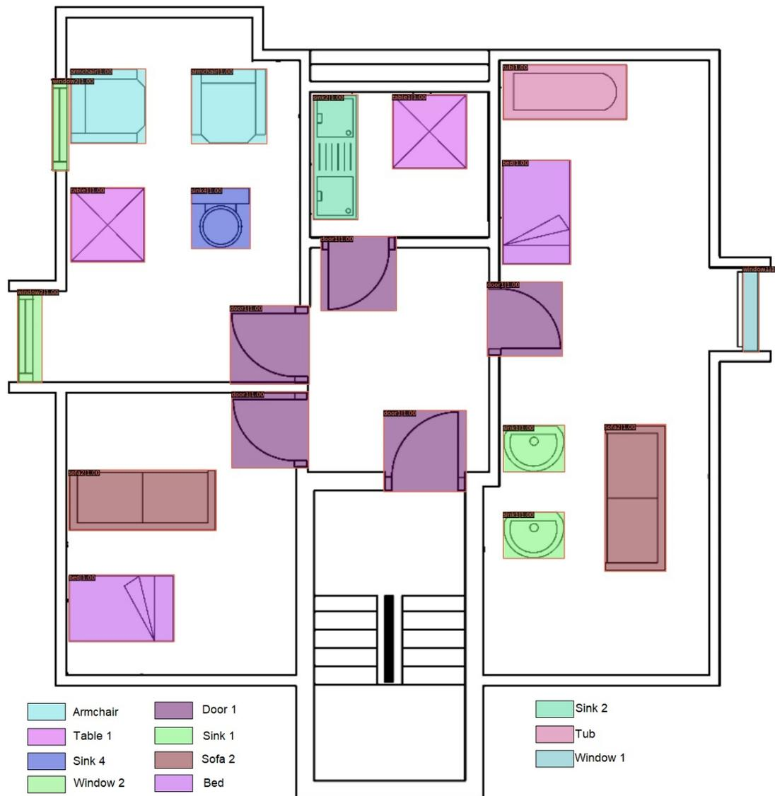
**Figure 10.** Sample output from experiment Our\_SFPI\_SESYD\_train\_SESYD\_test. It is evident that all furniture objects are identified and localized correctly.
