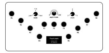
Figure 3: Hardware user interface, with eight actuator buttons (M1–M8), three function buttons (F1–F3), knobs to select the mode, slot, and amplitude, and the display.
