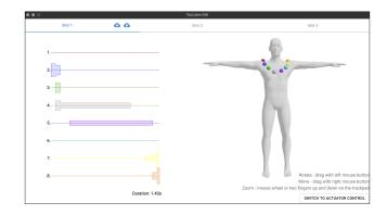
Figure 4: Screenshot showing the graphical user interface. A visualization of the pattern recorded by the *TactJam* hardware can be seen on the left. The positions of the actuators are manually indicated on the right, using this GUI.
