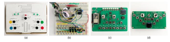
Figure 2: (a) Initial prototype of *TactJam* used for teaching, (b) breadboarded version of *TactJam* designed for TEI workshop, (c) first PCB version of workshop device and (d) re-designed workshop device with improved ergonomics for bimanual hand-held use.
