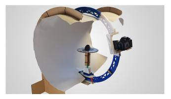
Figure 4: We used an open source photogrammetry rig that allows one to take a set of pictures from an object from different angles. These pictures were used in Meshroom to reconstruct 3D models of the climbing holds.
