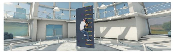
Figure 1: Virtual Reality rock climbing on a physical climbing treadmill. This allows for continuous climbing while wearing a head-mounted display. With the system presented in this work, we implemented different virtual scenarios. In this showcase application, the climber is placed into a virtual showroom.
