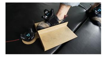
Figure 6: To visualize the hands and feet of the climbers, Vive trackers are attached to the climber's hands and feet. A spatially registered template is used for calibration, i.e. to align the virtual models to the physical trackers.
