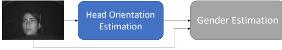
Fig. 2. Overview. The figure depicts the abstract idea of the proposed method. First, The head image is used to predict the head orientation. Afterwards, the face image, along with the predicted head orientation angles are fed into the gender estimation model.
