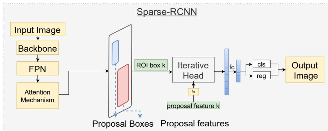
**Figure 4.** Flow diagram of page object detection with Sparse-RCNN in detail. Sparse-RCNN takes features from DyHead, and learns and proposes the optimal Region of Interest (ROI) boxes for the features, instead of a Region Proposal Network (RPN). The features are concatenated with latent proposal features, passed as FC layers, to predict and classify the objects.
