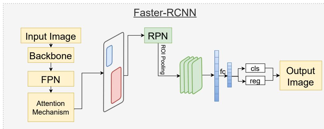
**Figure 3.** Flow diagram of page object detection with Faster-RCNN in detail. The features passed to the Faster-RCNN head initially passed through the Region Proposal Network (RPN) for generating proposal boxes of different dimensions. They are then aligned via ROI Pooling, to obtain fixed-size features. These features are then passed as fully connected layers (FC). Finally, the detected object is classified and a bounding box is computed.
