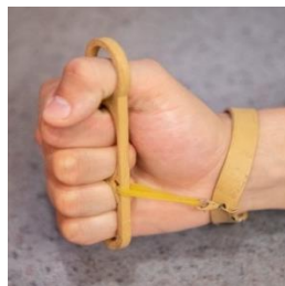
Fig. 18. The 3D printed hand spasticity disability simulation splint with an elastic band to replicate the clenched hand and wrist position of people with post-stroke upper limb spasticity
