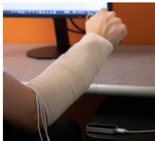
Fig. 2. The Leap Motion Controller (LMC) sensing a participant's fist position to control the cursor in a computer interface
