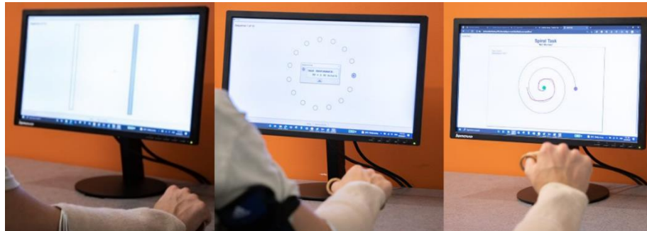
Fig. 3. From left to right, the one-dimension Fitts task performed by a participant using a conventional mouse, the two-dimension Fitts task and the spiral tracing task using the LMC
