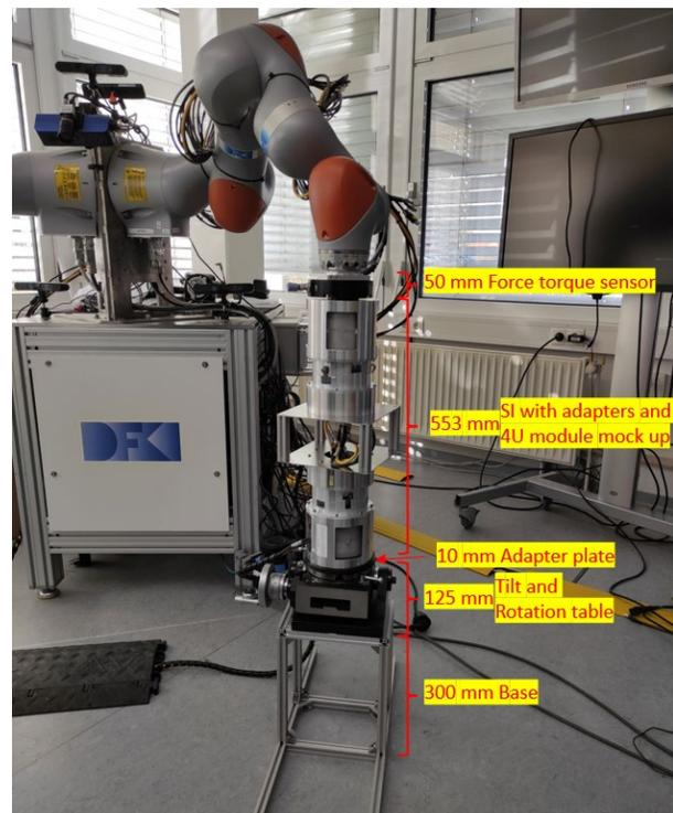
Fig. 7 Configuration and dimensions of the test setup.
