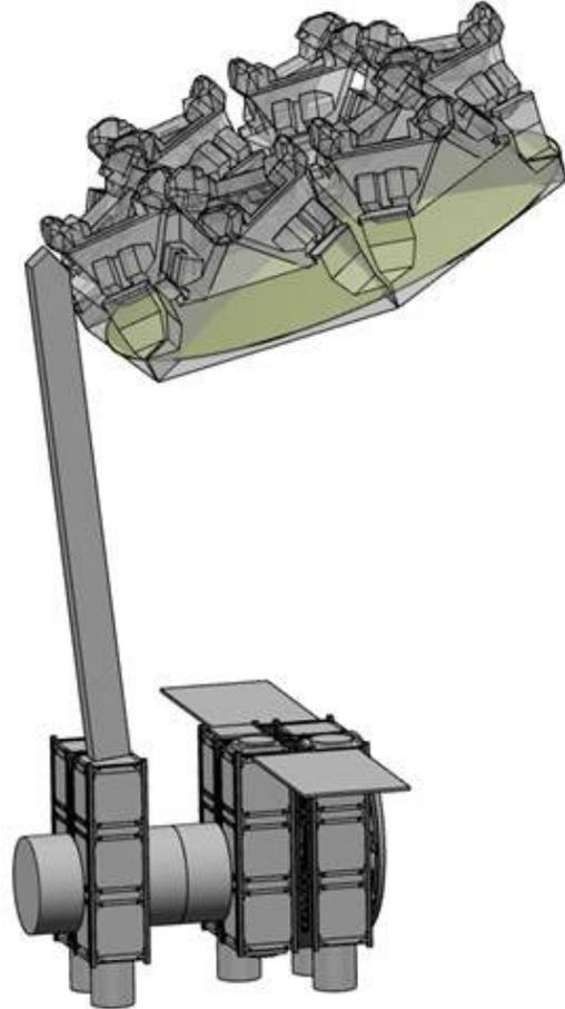
Fig. 2. CAD model of the fully assembled Client Satellite (credit: Airbus Defence and Space SAS).
