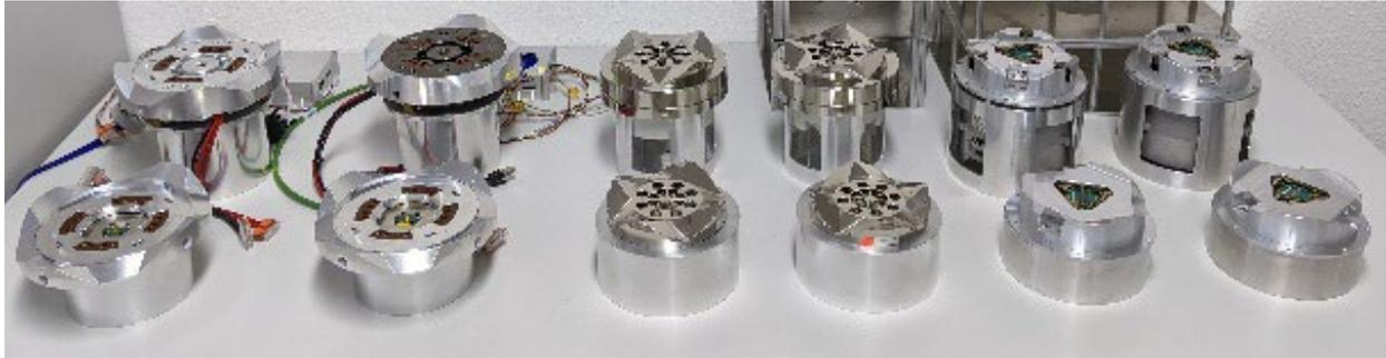
Fig. 6 In the context of the Project PERIOD with Benchmark tested SIs mounted on adapters from left to right: iSSI<sup>®</sup> active and passive with optional formfits [5], HOTDOCK active and passive [4] and SIROM active and passive [6]. The active type SI are in the back row and the passive SIs are in the front row.
