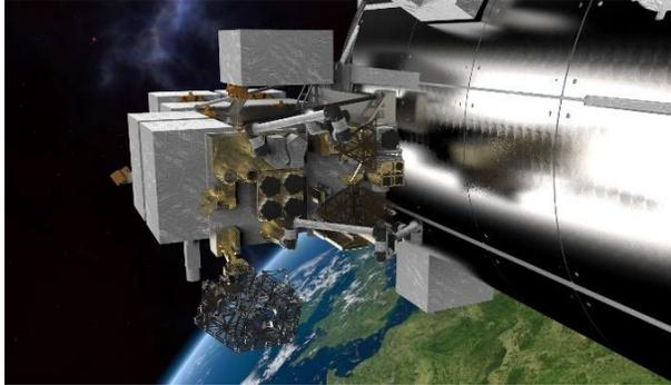
Fig. 1. The PERIOD Boxes mounted on the Bartolomeo platform outside of the Columbus module (credit: Airbus Defence and Space SAS).
