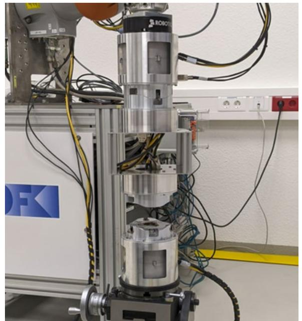
Fig. 10 Test setup with fixed payload module on the end-effector of the Kuka arm
