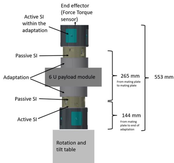
Fig. 8 Fixed distances of the test setup.
