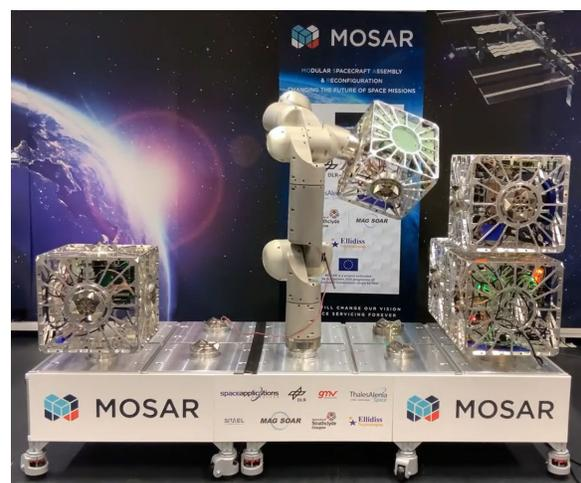
Fig. 3. MOSAR test setup with HOTDOCK for demonstration of spacecraft modules manipulation.
